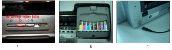
1) Press the "ink cartridge replace button" (Picture A) on the printer to move the cartridge to the cartridge remove position (Picture B).
