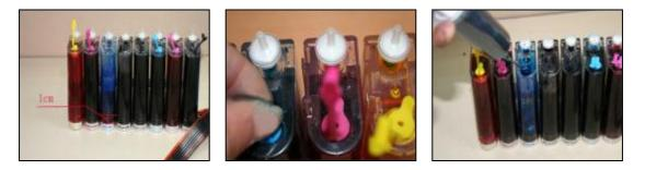
Please pay attention to the ink level in the reservoirs; if the ink level is below 1CM as the above picture shown, please use refill kits to fill ink into Reservoir bottles. Carefully pull out the rubber plugs from the refill holes.(there is possibility of ink spattering. Be careful!) Refill ink according to the color in short supply. Then put the rubber back. (Please keep the printer and the reservoir at the same horizontal line during the process of refilling ink.)
