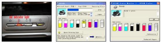
If the indicator light flashing when printing, it tells that you need to reset the chip to full status. Please turn off your printer for about 1 minutes and switch it back on. Ink meter bar shall show full ink. You can start printing as usual.
