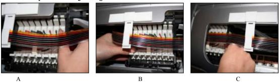
A. Adjust the length of the tube, move the cartridge Carrier
